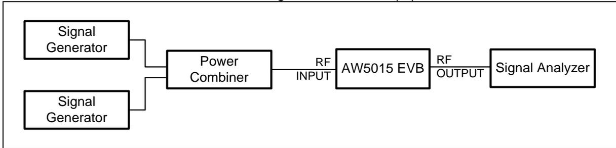
Figure 31. Circuit for intermodulation distortion test
