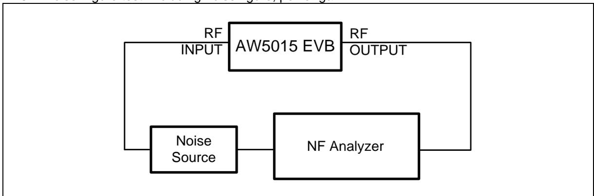
Figure 30. Circuit for Noise Figure test
